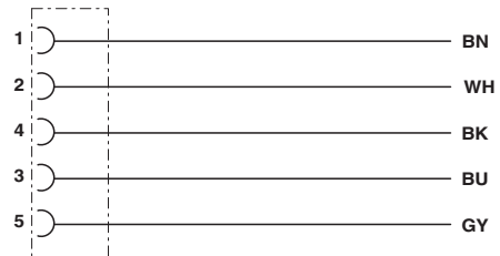
Contact assignment of the M12 socket
